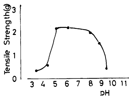
Figure 1. Effect of pH on the tensile strength of muscle fibers (g/25 single fibers)
